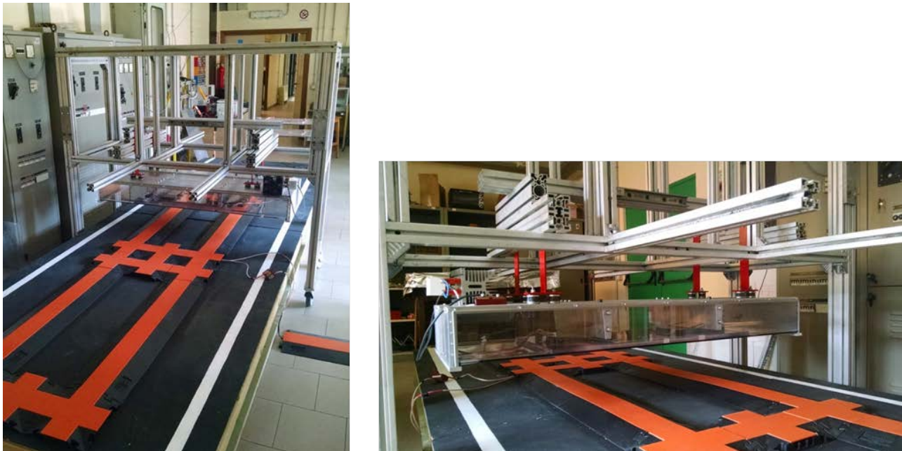
Figure 7.1 Prototypal structure for the laboratory test of the IPT CWD system
