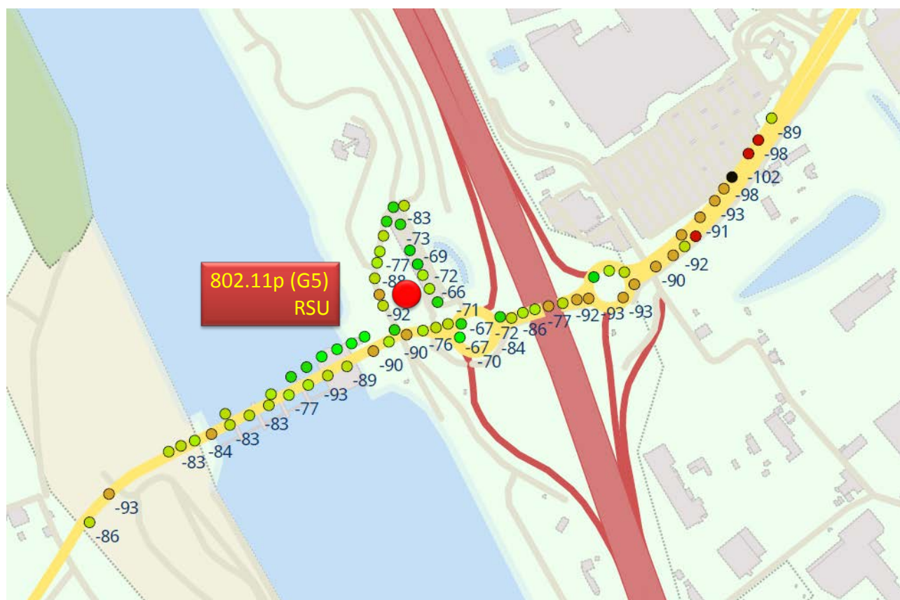
Figure 6.6. 802.11p (G5) radio signal levels at the test site
