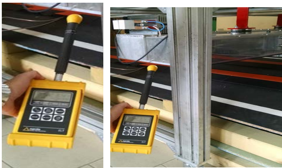
Figure 7.9 Measurement of the magnetic field induction during the functioning of the system
